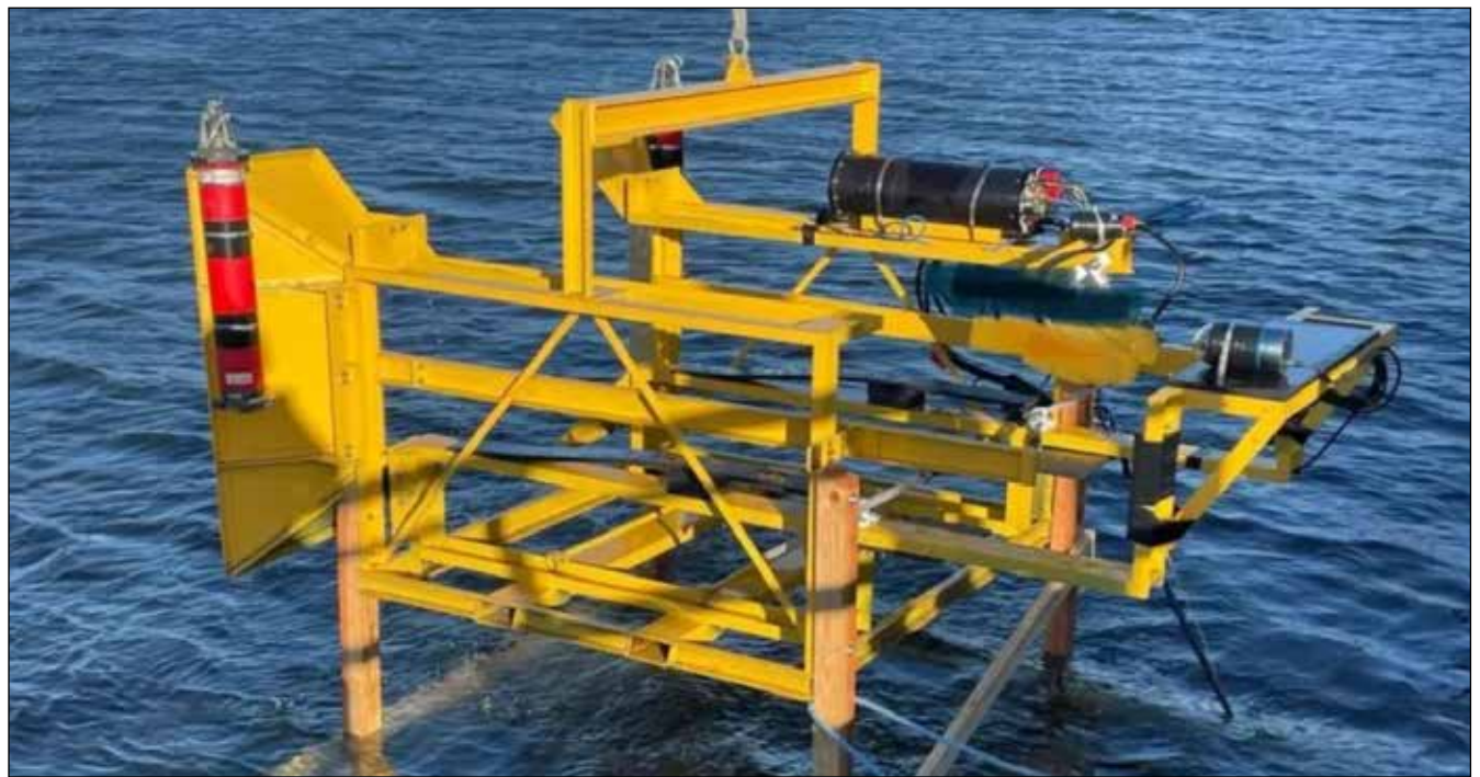
Autonomous vehicle docking stations allow the robots to recharge their batteries without human assistance. Credit: NOAA
